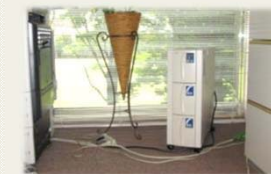
Portable storage battery of IIF Shinonome R&D Center
